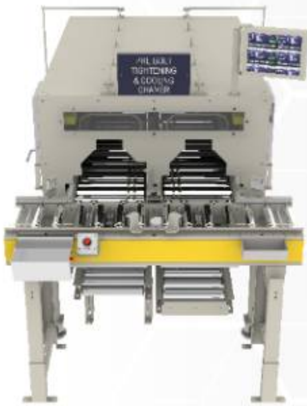
Cooling Chamber CV & Pre Bolt Station
